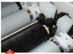
Brush in rinse section to ensure plates are thoroughly cleaned before gumming.
