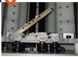
Heavy duty belt drive system with AC drive and brush motors for near maintenance free operation.
