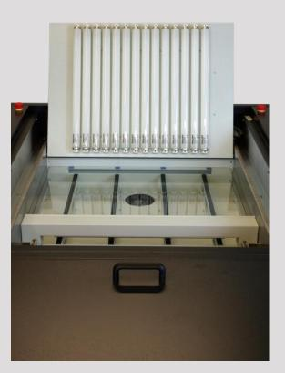
**Plate Mounting:** Plate mounting is by means of a stainless steel carrier sheet. Affixed to the carrier sheet smooth plastic mounting material and Tessa double sided tape for Mylar/Polyester backed plates or a magnetic self-adhesive sheet for steel backed plates (Dry Offset). The plate is affixed to the carrier sheet and positioned onto the input table. The MANTA automatically starts the plate production cycle by means of an inductive sensor.
