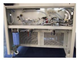
Easy access to all major components including pumps and motors via quick release and removeable covers
