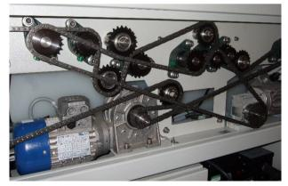
Heavy duty chain drive system with AC drive and brush motors. Idlers fitted with sealed ball race bearings for maintenance free operation
