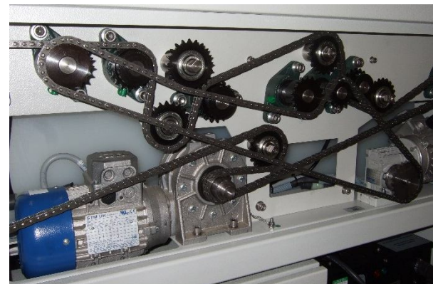
Heavy duty chain drive system with AC drive and brush motors. Idlers fitted with sealed ball race bearings for maintenance free operation
