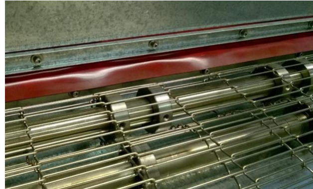
Self-contained internal wire conveyor belt with silicone rubber curtains on entry & exit to ensure minimal heat loss and to reduce power consumption
