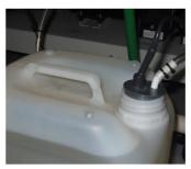
the developer replen bottle is empty, or the developer overflow bottle is full.
