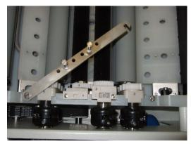
All rollers easily removed for cleaning and maintenance
